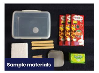
The above tub was approx. 230mm by 170mm (2litre capacity) and required 5½ packs of plasticine for a 10mm deep layer. Two packets of jelly making approx. 1 litre, gives a sufficient depth of "unstable ground".
